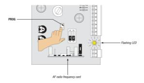
2) The transmitter button sends the code, and the LED will stay on to signal that memorisation was successful.
